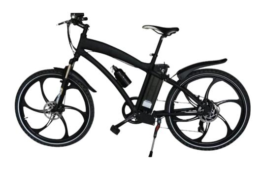
Motor:500W integrated wheel motor
