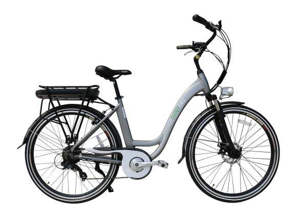
• Motor: 250W hub motor with water proof connector
